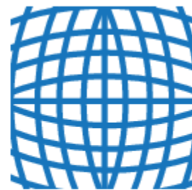
Positive radial distortion "barrel"
